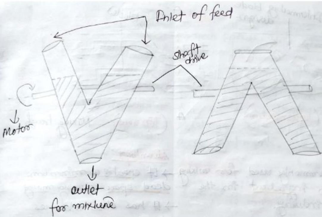
Uses : → Used for solid mixing.
