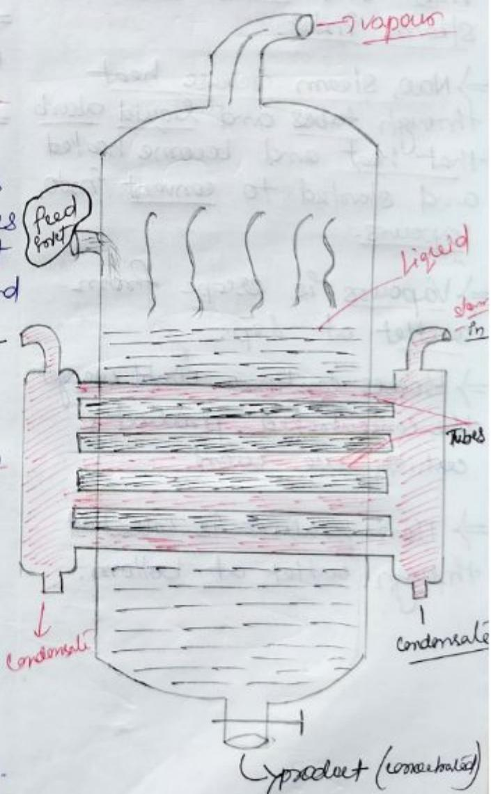
→ Steam inlet from which steam enters also condensate for steam and outlet for steam
